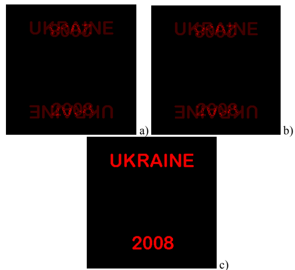
Fig. 2. Images restored from Fourier hologram (a), Hilbert hologram (b) and combined hologram (c).
