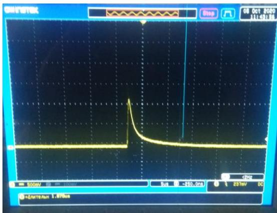
**Fig. 3.** Oscillogram of the photodetector signal corresponding to the laser output energy 25  $\mu$ J.
