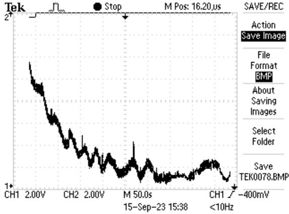
**Fig. 7.** Oscillogram of the voltage on the measurement resistor demonstrates the degradation process of the elastic contact: current flows from a +30 V source through the nanofilm and a 10 MOhm resistor; the measurement duration is 7 min; at the beginning, the current is  $1.1 \pm 0.05 \mu\text{A}$ ; after 3 min of observation, the current decreases to  $200 \pm 50 \text{ nA}$  and continues to decrease.
