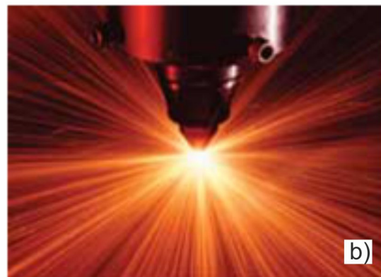
Fig. 2. 3015/4020 type optical fiber laser cutting machine (a) and its cutting head in operation mode (b).
