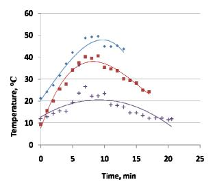
Experimentally obtained dependences of the battery temperature on the time of discharge:  $\blacklozenge$  – in the laboratory at the temperature 22 °C,  $\blacksquare$  – outdoor at the temperature 8 °C, + – outdoor at the temperature 4 °C.
