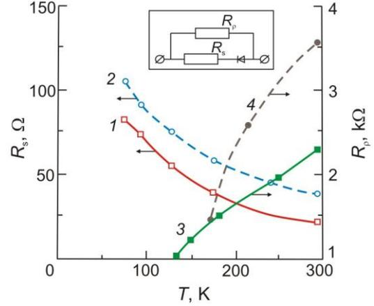
**Fig. 4.** Temperature dependences of the  $\text{GaAs}_{1-x}\text{P}_x$  orange parallel ( $R_p$ ) and series ( $R_s$ ) resistances for initial (1) and irradiated by 2 MeV electrons: 2 –  $F = 2.64 \cdot 10^{16} \text{ cm}^{-2}$ , 3 –  $2 \cdot 10^{14} \text{ cm}^{-2}$ , 4 –  $9.5 \cdot 10^{15} \text{ cm}^{-2}$ .
