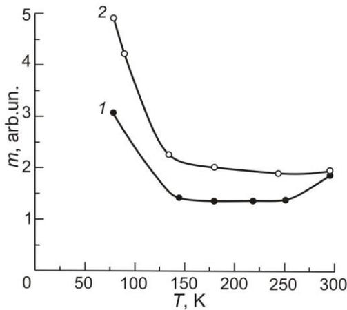
**Fig. 3.** Temperature dependence of the non-ideal coefficient  $m$  in irradiated orange  $\text{GaAs}_{1-x}\text{P}_x$  LED: 1 –  $F = 2 \cdot 10^{14} \text{ cm}^{-2}$ , 2 –  $F = 9.5 \cdot 10^{15} \text{ cm}^{-2}$ .
