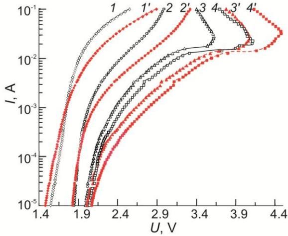
**Fig. 2.** Current-voltage characteristics of the orange  $\text{GaAs}_{1-x}\text{P}_x$  diode in the mode of the current generator at different sample temperatures: initial: 1 – 300 K, 2 – 180 K, 3 – 95 K, 4 – 77 K; irradiated ( $E = 2 \text{ MeV}$ ,  $F = 2.64 \cdot 10^{16} \text{ cm}^{-2}$ ): 1' – 300 K, 2' – 180 K, 3' – 95 K, 4' – 77 K.
