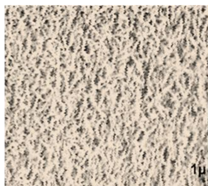
Fig. 2. SEM micro-image of the surface of 190-nm thick vacuum deposited PbPc thin solid film.
