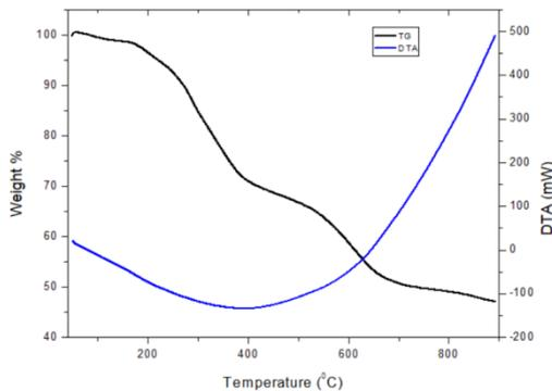
**Fig. 9.** TGA/DTA graph of AgO NPs.
