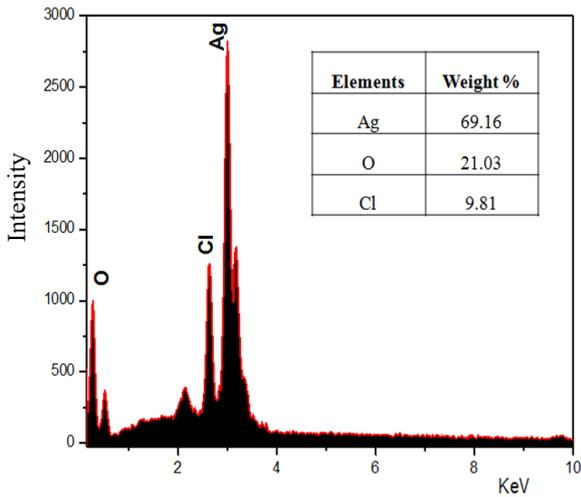
Fig. 6. EDX spectrum of AgO NPs.
