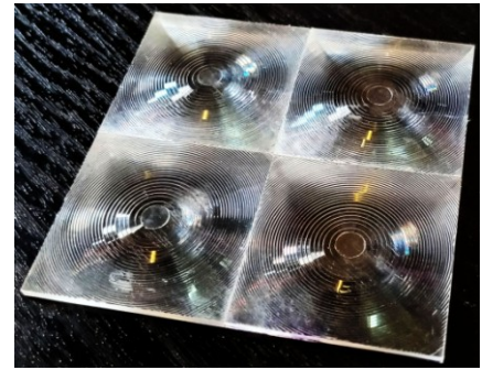
Fig. 13. Image of a diagnostic module consisting of four apertured lenses #32-c1-#(07-10).
