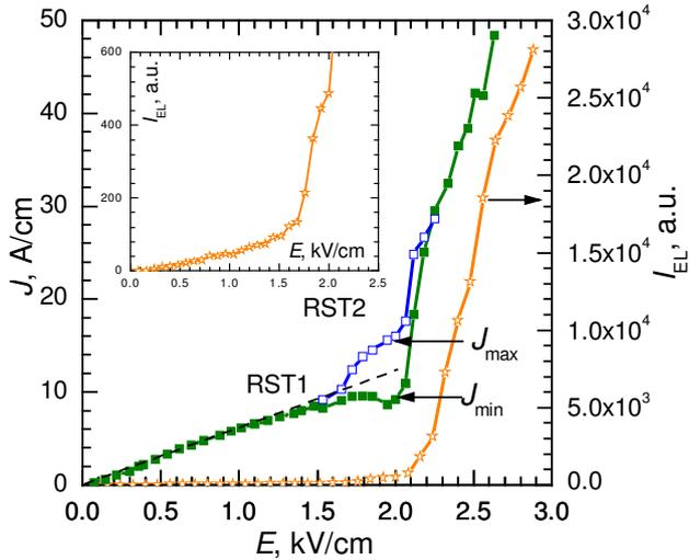
**Fig. 3.** Field dependence of the current and integrated EL intensity. The maximum ( $J_{\max}$ ) and minimum ( $J_{\min}$ ) current values are shown for the current oscillations. Inset: the field dependence of the integral radiation intensity in the smaller scale.  $T = 4.2$  K.
