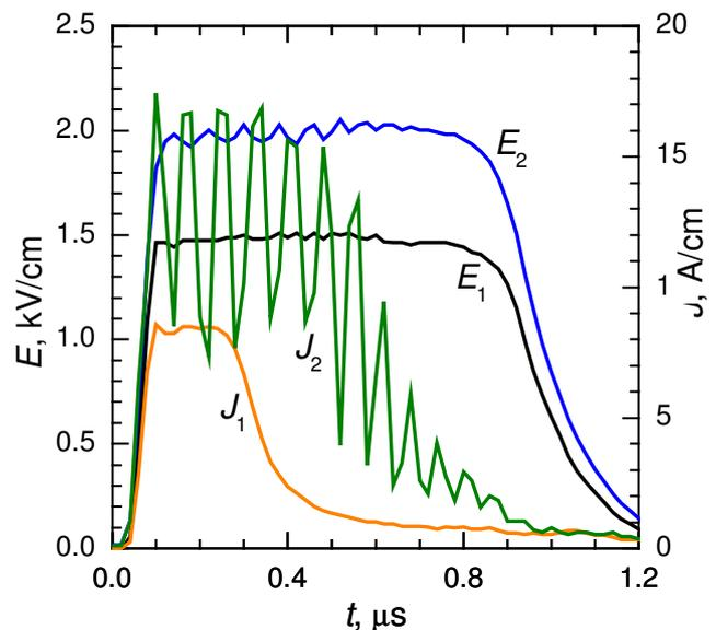
**Fig. 2.** Waveforms of pulses for the applied field and current.  $E_1 = 1.45$  kV/cm, and  $E_2 = 1.9$  kV/cm.  $T = 4.2$  K.
