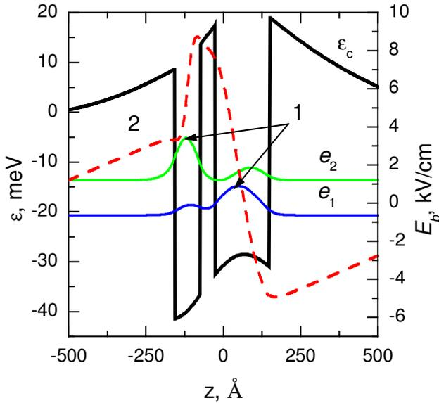
**Fig. 1.** Potential profile of the conduction band bottom  $\varepsilon_c$  for the structure (one period); the bottom energies of lowest electron subbands  $e_i$  and squared envelope wave functions of electrons ( $I$ ). Dashed line indicates the distribution of the built-in electric-field  $E_b$  (2).  $T = 10$  K.
