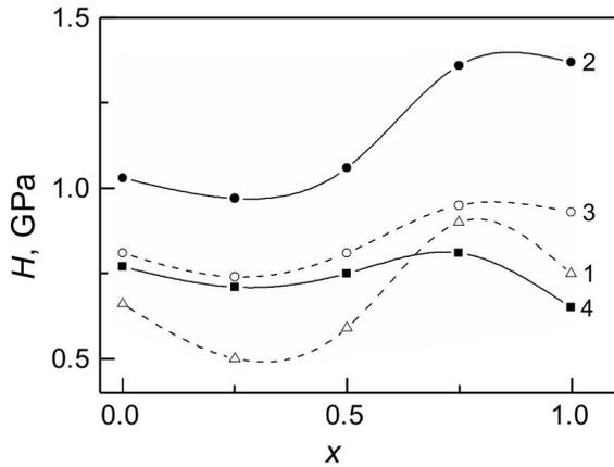
**Fig. 1.** Compositional dependences of mechanical parameters for  $(\text{Cu}_{1-x}\text{Ag}_x)_7\text{GeS}_5\text{I}$  mixed crystals: (1) micro-hardness  $H$ , (2) maximal value of micro-hardness  $H_{\max}$ , (3) micro-hardness  $H_{200}$  at the load force  $P = 2$  N, (4) hardness  $H_0$  at an infinite depth of the imprint (obtained when extrapolating  $H(h)$  in the plastic deformation gradient model (MSG)).
