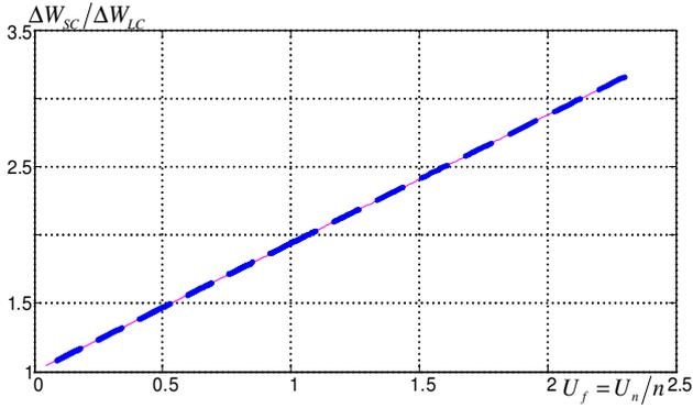
**Fig. 3.** The ratio of energies accumulated in SC and LC for the time of charge to the value of the final voltage on the terminals of capacitors  $\frac{\Delta W_{SC}}{\Delta W_{LC}}\left(\frac{U_n}{n}\right)$ .
