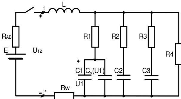
Fig. 1. Equivalent scheme of SC.
