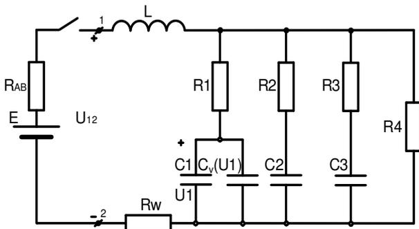
Fig. 1. Equivalent scheme of SC.
