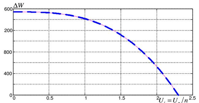
**Fig. 4.** Dependence of the difference between energies  $\Delta W$  accumulated in SC and LC, in the process of charge from the initial voltage  $U_f = U_n/n$  up to the final voltage  $U_f = U_n$ .
