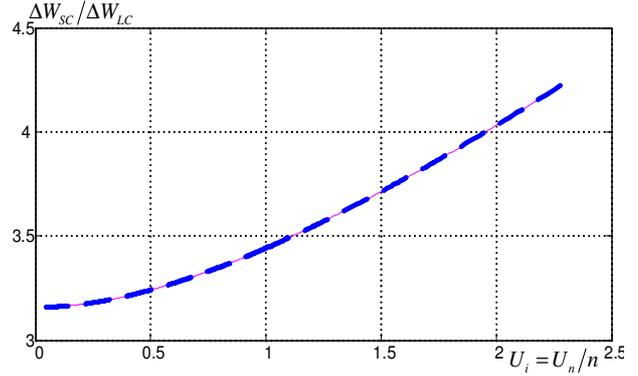
**Fig. 5.** Dependence of the ratio of energy doses accumulated in SC and LC during the charge from the voltage  $U_i = U_n/n$  to  $U_f = U_n$  on the value of initial voltage on the terminals of capacitors.
