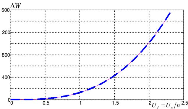
**Fig. 2.** The dependence of the influence of finite conditions under the voltage on terminals of the capacitors  $U_f = U_n/n$  on the difference in the energies  $\Delta W$  accumulated in SC and LC.
