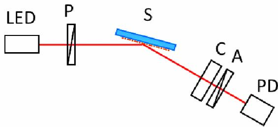
Fig. 2. Optical circuit for polarimetric measurements. LED – source of radiation, P – polarizer, S – sample, C – compensator (quarter-wave phase plate), A – analyzer, PD – photodetector.
