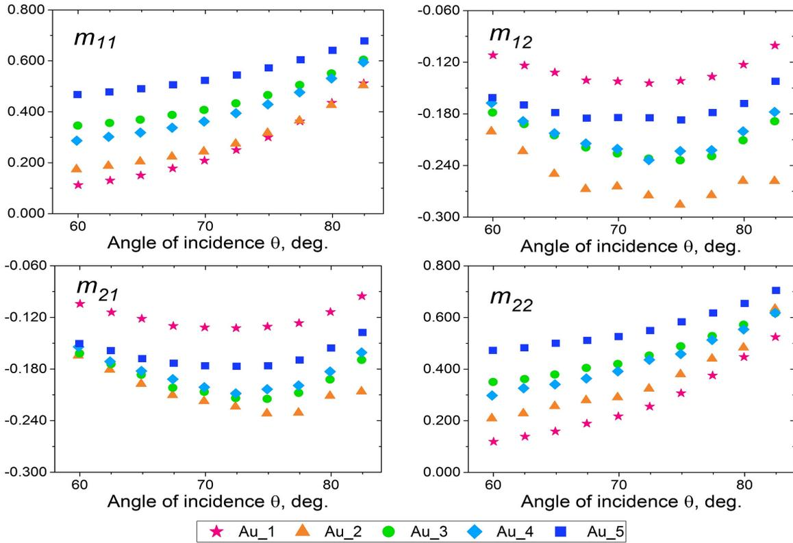
**Fig. 3.** Angular dependences for elements of upper left minor of the Mueller matrix of studied samples of island films.
