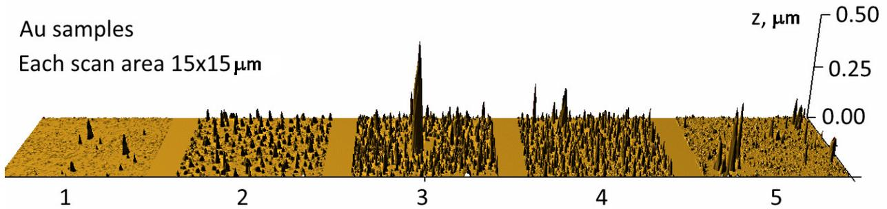
Fig. 1. AFM-images of a set of 5 samples of island gold films.
