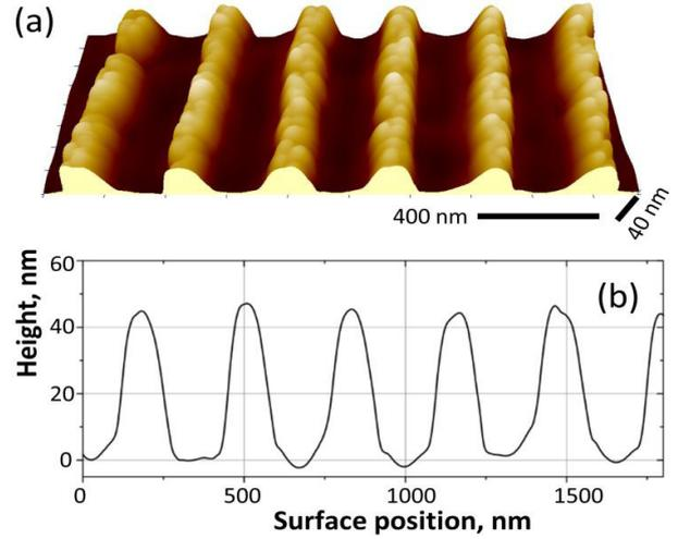
**Fig. 1.** AFM image (a) and cross-section (b) of the Au grating with spatial frequency of  $3370 \pm 5 \text{ mm}^{-1}$  and average value of slit width between nanowires is about 150 nm.
