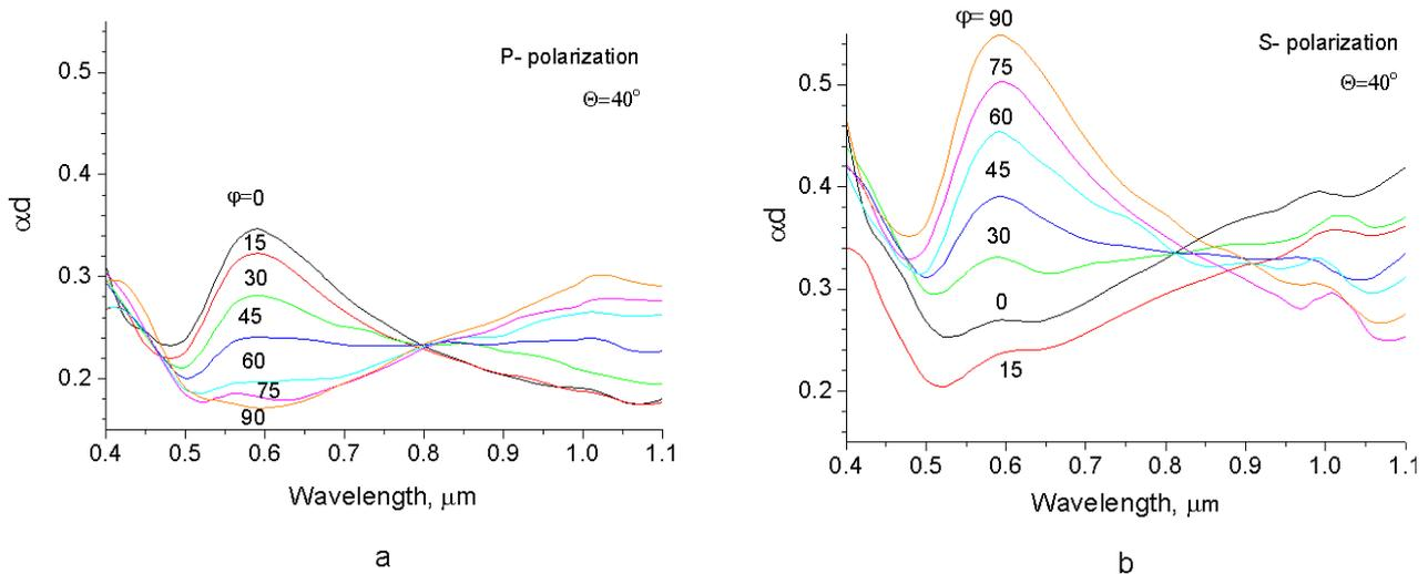
**Fig. 3.** Spectra of extinction ( $ad$ ) at the azimuthal angles from 0 to 90° with the step 15° for  $P$ -polarized (a) and  $S$ -polarized (b) light. The angle of incidence ( $\theta$ ) is 40°. The sample with the average slit width between nanowires close to 150 nm.
