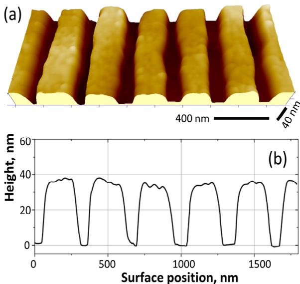
**Fig. 4.** AFM image (a) and cross-section (b) of the Au grating with the spatial frequency  $3370 \pm 5 \text{ nm}^{-1}$  and minimal value of slit width between nanowires (average slit width is about 40 nm).
