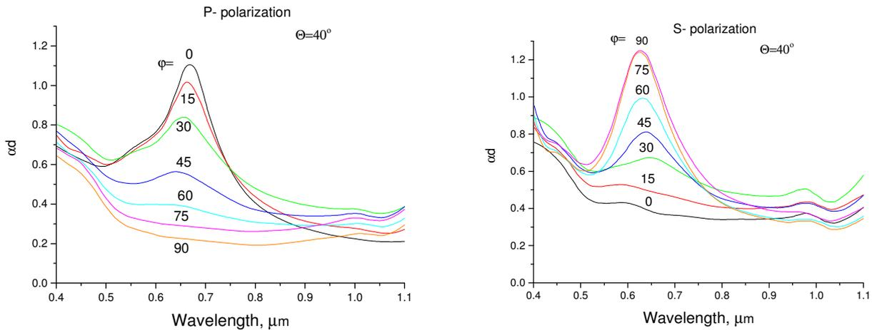
**Fig. 6.** Spectra of extinction ( $ad$ ) at the azimuthal angles from 0 to 90 with the step  $15^\circ$  for  $P$ -polarized (a) and  $S$ -polarized (b) light. The angle of incidence ( $\theta$ ) is  $40^\circ$ . The sample with the average slit width between nanowires close to 40 nm.
