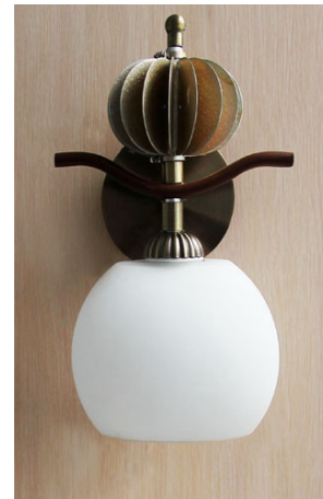
Fig. 3. The appearance of the sample lamp with a cooling system based on heat pipe.
