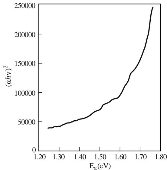
**Fig. 3.** Spectral dependences of the absorption near the energy gap  $(\alpha h\nu)^2 \rightarrow E_g$  of  $\text{MoRe}_{0.001}\text{Se}_{1.999}$ .
