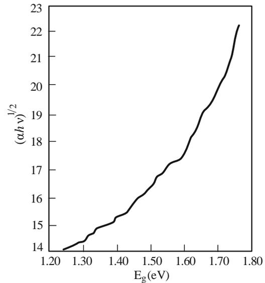
**Fig. 4.** Spectral dependences of the absorption near the energy gap  $(\alpha h\nu)^{1/2} \rightarrow E_g$  of  $\text{MoRe}_{0.001}\text{Se}_{1.999}$ .
