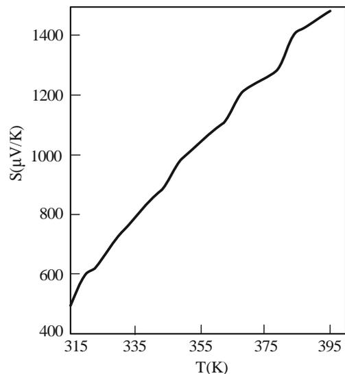
Fig. 2. Seeback coefficient ( $S$ ) (in  $\mu\text{V/K}$ ) of  $\text{MoRe}_{0.001}\text{Se}_{1.999}$ .
