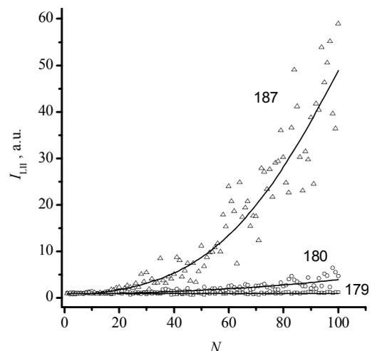
**Fig. 1.** Silicon surface LII intensity as a function of irradiation dose, where  $N$  is the number of laser pulses. Numbers near the curves indicate the laser surface power density in MW·cm<sup>-2</sup>.
