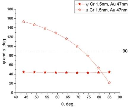
**Fig. 3.** Angular dependences of parameters  $\psi$  and  $\Delta$  for the Au (reference) sample.
