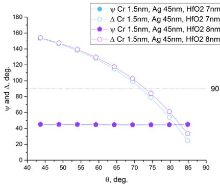
**Fig. 4.** Angular dependences of parameters  $\psi$  and  $\Delta$  for Ag-based samples.
