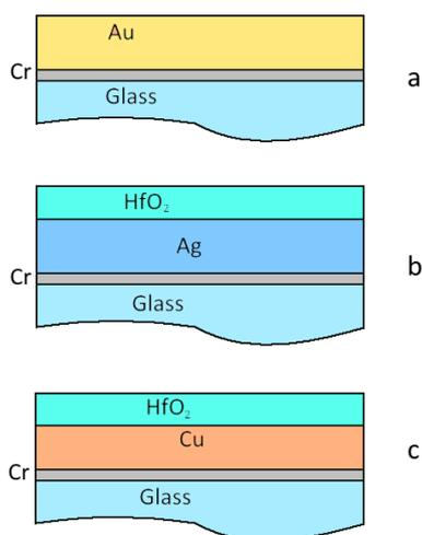
**Fig. 1.** Hybrid multilayer structure of the investigated samples based on Au (a), Ag (b) and Cu (c) thin films.
