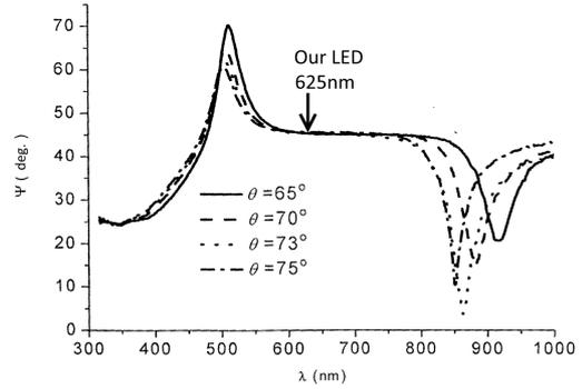
**Fig. 7.** Spectral dependences of ellipsometric parameter  $\psi$  of the heterostructure Cr (3 nm), Au (30 nm), HfO<sub>2</sub> (45 nm) for different angles of light incidence.
