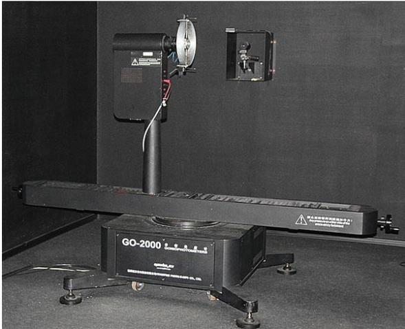
Fig. 5. Lighting device mounted on GO-2000 goniometer.
