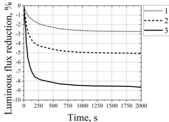
**Fig. 4.** Time dependence of luminous flux for different values of LED matrix power supply current: 1 – 1 A, 2 – 2 A, 3 – 3.5 A.
