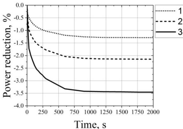
**Fig. 3.** Time dependence of electric power for different values of LED matrix power supply current: 1 – 1 A, 2 – 2 A, 3 – 3.5 A.
