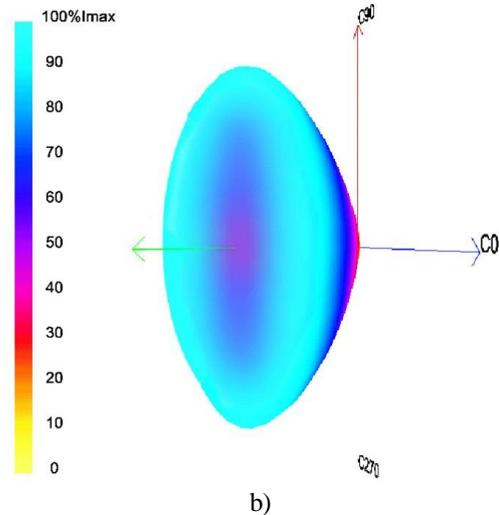
Fig. 6. Luminous intensity distribution curve for the C0/180 plane (a) and 3D photometric body visualization of the lighting device (b).
