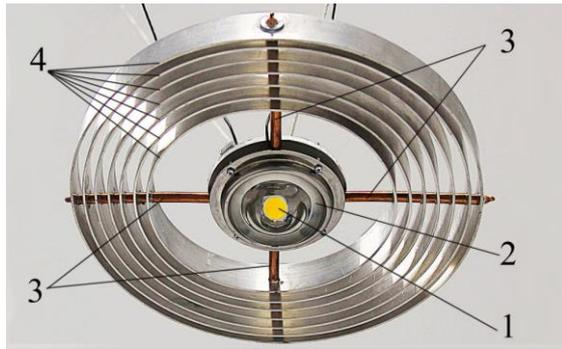
**Fig. 1.** LED lighting device: 1 – LED matrix, 2 – lens, 3 – heat pipes, 4 – elements of heat exchange with ambient air.
