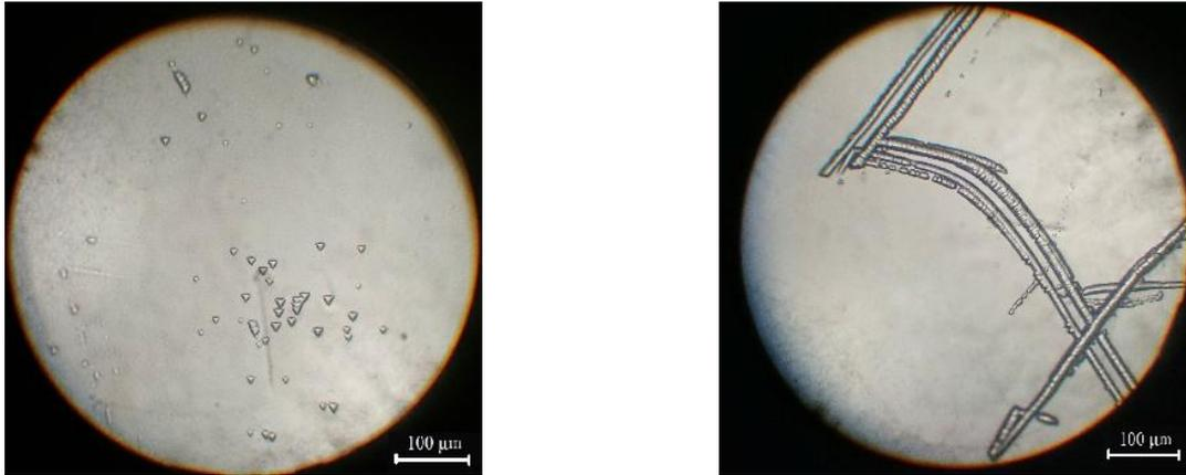
**Fig. 6.** Dislocations at the depth 24  $\mu\text{m}$  in the silicon wafer.
