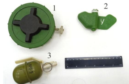
Fig. 3. Photos of the simulants used in the experiments: 1, 2 – reduced plastic models of AP mines ПМН-2 and ПФМ-1, respectively, 3 – training simulation grenade ПИПО-5Г.
